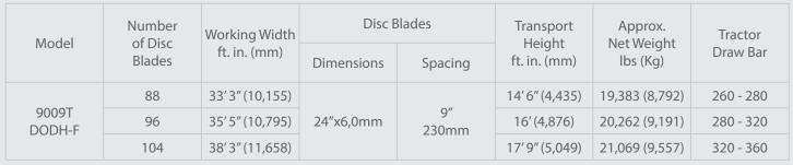
> Transport Width: 17'9" | Avg. Weight per Disc: 192 lbs (87 Kg) | Axle Diameter: 1.3/4"
